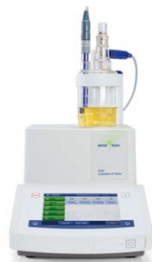
Water determination by Karl Fischer Titration
