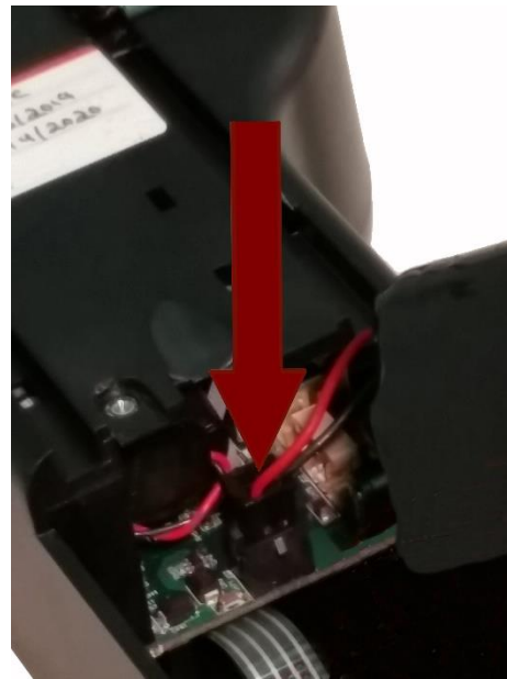
Step 4 – Insert battery connector plug into matching socket on PCB board in battery compartment
