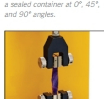
TA-GPJ General Peeling Jig measures the adhesive strength needed to remove the lid from a sealed container at 0°, 45°, and 90° angles.
