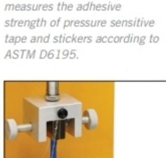
TA-LTT Loop Tack Test measures the adhesive strength of pressure sensitive tape and stickers according to ASTM D6195.
